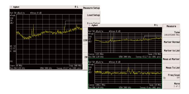
Setting up the E7400A Series EMC analyzer is completed in three easy steps: (1) select the band for the test; (2) choose the limit line; and (3) select the correction factors for the transducers, cables, and amplifiers.
